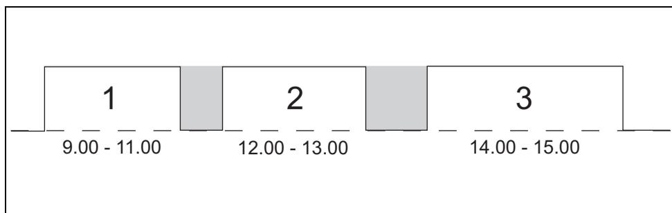
*The machine switches on at 9.00/12.00/14.00 automatically. The machine is on stand-by at 11.00/13.00/15.00. During stand-by mode the control panel is switched off and the boiler temperature drops to the set boiler temperature.*
